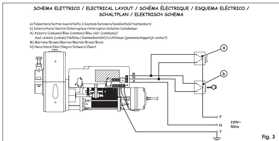
**SCHEMA DI APPLICAZIONE DEL KIT ELETTROFRENO / INSTALLATION LAYOUT FOR
