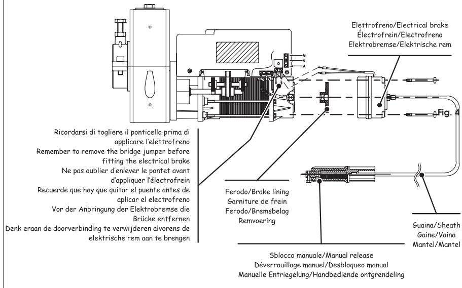
**VISTA ESPLOSA DEI COMPONENTI DEL GRUPPO ELETTROFRENO / EXPLODED VIEW OF
